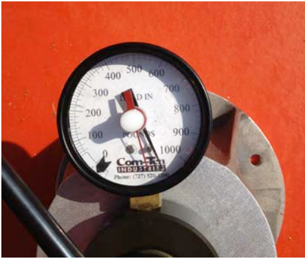
Typical Adhesion Testing Results Pull test results of over 1,000 PSI, exceeding the capacity of the test apparatus, were typical.
